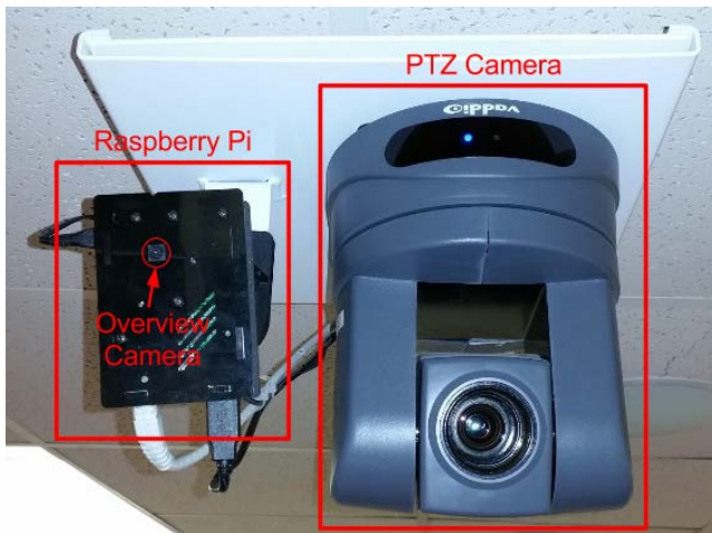
Figure 1: PTZ implementation using a Raspberry Pi
