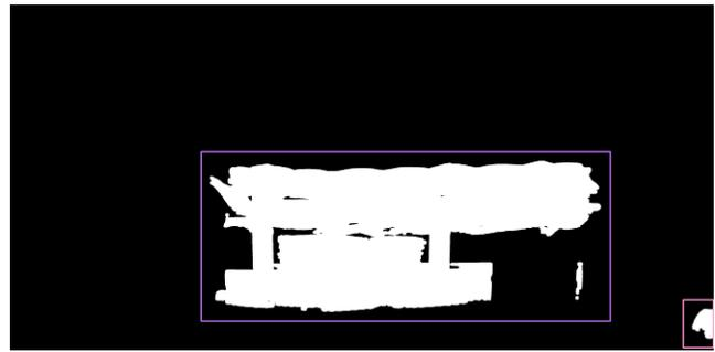
**Figure 7 - Binary Image Showing all Motion Merged and Bounded with Rectangles**
