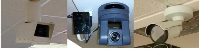
**Figure 1 - From Left: Static Camera, PTZ Camera, 4K Camera**
